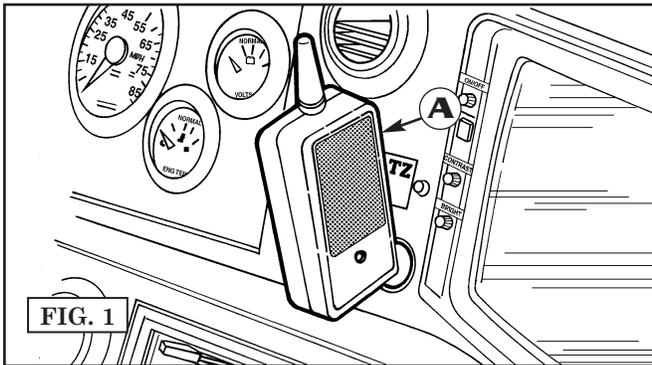
The **Receiver** (Fig. 1 / **A**) plugs into a 12-volt outlet on the dash of the motorhome. A red indicator light will illuminate once. A green LED light will illuminate and stay on indicating a good continuity power source. When the BrakeBuddy is activated in the towed vehicle, the Receiver will illuminate.
