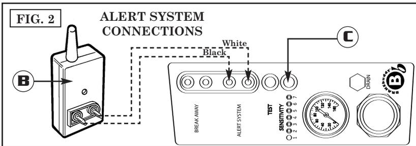
The **Transmitter** (Fig. 2 / **B**) plugs into the top of the BrakeBuddy and sends a signal to the Receiver when the BrakeBuddy is activated. Plug the transmitter into the connections on the BrakeBuddy marked "Alert System" (Fig. 2). The antennae should point towards the motorhome.
