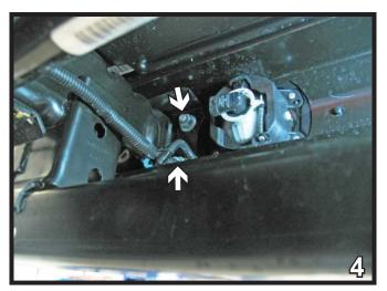
4. Using a 18mm socket, remove the two (2) bolts on inside edge of frame. Do this on both sides of the the vehicle.
