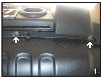
Using a Phillips screwdriver, remove the four (4) push pins from the bottom of the belly pan. There are two (2) on each side.
