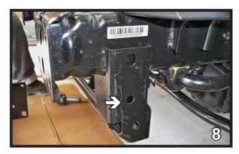
8. On the 2010 models and newer: Align the baseplate's lower hole with the existing middle hole in the frame, insure baseplate is level with frame and clamp in place with the vice grips. Do this to both sides of the vehicle.
