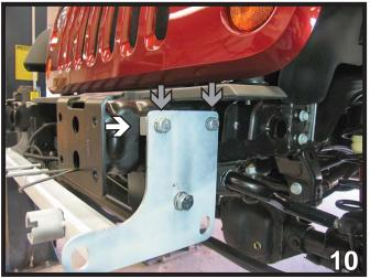
10. Using a 17/32" drill bit, drill the top holes of the baseplate thru the frame. Install the spacer plate in between the baseplate and frame (white). Install 1/2"-13 x 1-3/4" bolts with 1/2" lock washers thru the baseplate, spacer and frame (gray). Insert 1/2" whiz nuts with wires on the inside of the frame. Do this on both sides of the vehicle.
