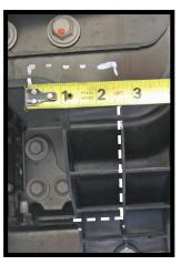
8. Using a reciprocating saw, trim an area on the frame approximately as shown. Cut the bottom flush with the bottom rail (gray) and vertically just inside the rib (approximately 1-5/8") then 2-1/2" back at the top. Do this on both sides of the vehicle.
