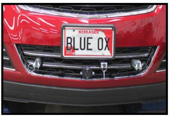
15. Hold the fascia as close to its original postion, mark and trim the fascia around the convienence links and attachment tabs. Reinstall the fascia and fascia shroud.
