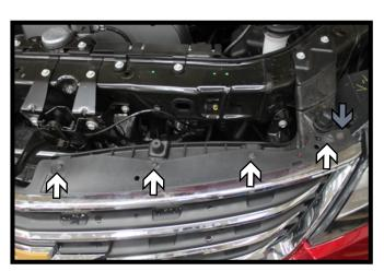
2. Using a T20 Torx, remove the seven (7) screws from the top edge of the fascia (white). There are four (4) on the driver side and three (3) on the passenger side. Using a 7MM socket, remove the two (2) screws from the top edge of the fascia corners (gray). There is one (1) on each side of the vehicle.
