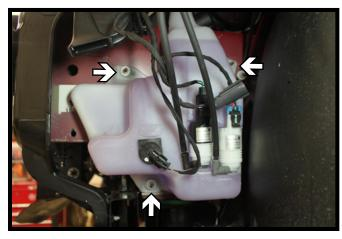
On the driver side, using a 10MM socket, remove the three (3) nuts from the washer fliud reservoir. Disconnect all lines and electrical connections, then set reservoir aside.
