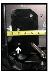
9. Tip the baseplate onto the frame. Measure down 2-13/16" from the top of the frame to the top of the baseplate. Measure 6-1/4" from the front of the frame to the back of the baseplate. Level the baseplate and clamp into position. Using the baseplate as a template, drill a 13/32" hole (white) and insert a 3/8"-16 x 1" hex bolt, 3/8" lock washer and 3/8"-16 hex nut. Do this to both sides of the vehicle. Tighten down fasteners.
