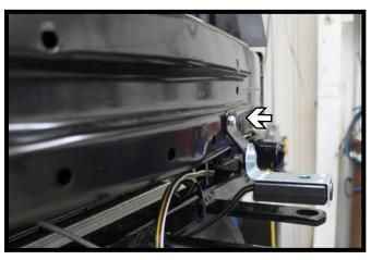
14. Optional: Attach the breakaway bracket to the metal bumper with the #10-16 x 1" self drilling screw at the desired location. Attach the breakawy to the bracket with a 1/4"-20 x 3/4" bolt and 1/4"-20 whiz nut.
