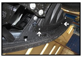
4. On the underside of the fascia, using a T20 Torx, remove the outer screws (white). Then using a 10MM socket, remove the inner screw (gray). Do this on both sides of the vehicle. Disconnect all electrical wiring and remove the fascia from the vehicle.
