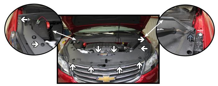
Remove the ten (10) push pins from the top edge of the fascia shroud (white). Then pry up the ends of the rubber strip on each side, releasing the clip underneath (gray). Remove the shroud from the vehicle.
