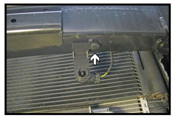
On the driver side, remove the push pin from the temperature sensor and temporarily move above the bumper. The sensor will be relocated later.
