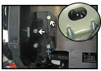
10. Drill out remaining holes with a 13/32" drill bit. Insert a 3/8"-16 x 1" hex bolt, 3/8" lock washer and 3/8"-16 hex nut in the other bottom hole (gray). In the top two (2) holes (white), install 3/8"-16 x 1-1/2" hex bolts and 3/8" lock washers attached to 3/8"-16 nut plates inserted up inside the bottom of the frame. Do this to both sides of the vehicle.
