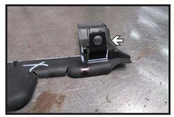
14. Remove the temperature sensor holder from the removed driver side plastic piece to be reinstalled on the vehicle.
