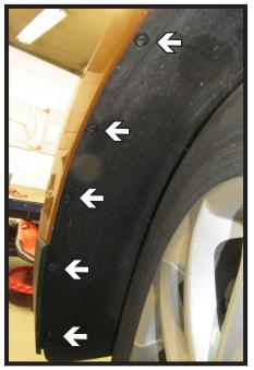
2. Using a T15 Torx, remove the five (5) bolts from along the edge of the wheel well. Do this on both sides of the vehicle.
