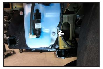
16. Reinstall the windshield washer fluid reservoir using existing hard ware except for the indicated bolt, use the 6MM bolt and 1/4" flat washer provided to attach to the baseplate. Reconnect all lines. Reinstall driver side headlight.
