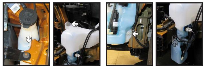
7. Using a 10MM socket, remove the three (3) bolts (white arrows) and one (1) nut (gray arrow) holding the windshield washer reservoir. Unplug all lines and set aside to be reinstalled later.
