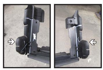
13. Using a utility knife, trim the indicated areas from the plastic piece before reinstalling to the front of the grill using existing push pins.
