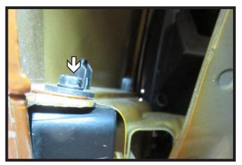
3. Pull back the wheel well liner. Then using a 7MM socket, remove the bolt from inside the wheel well. Do this for both sides of the vehicle.
