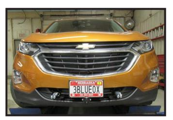
Hold the fascia as close to its original position, mark and trim the fascia around the convenience links and attachment tabs. Reinstall the fascia.
