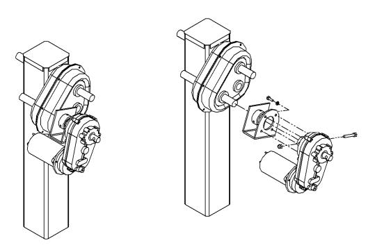
**Dual Leg Application**-The El Pac 2 can be used in a dual leg application. When properly mounted, this unit has a maximum lifting capacity of 6500 lbs. of combined jack weight. Due to the additional linkage required to add a second jack, and the possible misalignment of the jacks, you could experience a loss of lifting capacity in the 10% range.
