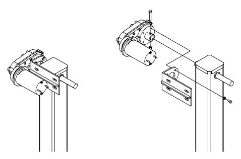
**Dual Leg Application**-The El Pac 1 must be installed on the passenger side of the passenger side jack leg in a dual leg application. When properly mounted, this unit has a maximum lifting capacity of 5000 lbs. of combined jack weight. Due to the additional linkage required to add a second jack, and the possible misalignment of the jacks, you could experience a loss of lifting capacity in the 10% range.
