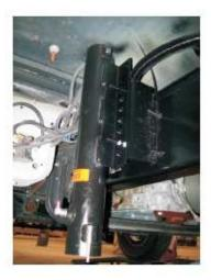
Once the cylinder is installed you will want to locate the (2) 90 degree elbow fittings (supplied). One will attach to the bottom or "retract" port. For the top you have a choice of the left or right port, use the side that keeps the hose from binding or pinching.
