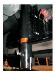
Completed corner with hoses and feet installed.
