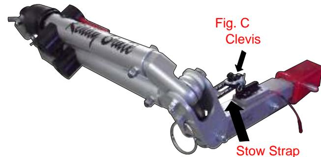
**(Note)** If RV is to be driven with tow bar in stow position NSA recommends wrapping legs with bungee strap, and hooking leg ends to RV bumper to hold Ready Brute in place over rough roads.
