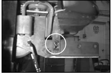
8. Remove top bumper bolt on each side and install brace with 8mm x 1.25 x 25mm bolt, 8mm lockwasher, and 8mm fender washer. Secure bottom of brace to frame mount using 3/8" x 1" bolt (circled above), 3/8" lockwasher,3/8" flatwasher, and 3/8" hex nut. We require that "L@CTITE. Blue" be used on all bolts.
