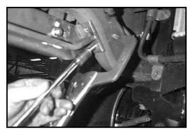
9. Install self-threading bolts at this time, and tighten all previously mentioned hardware to proper torque specifications. Remove C-clamps We require that "L@CT/TE.Blue"be used on all bolts.
