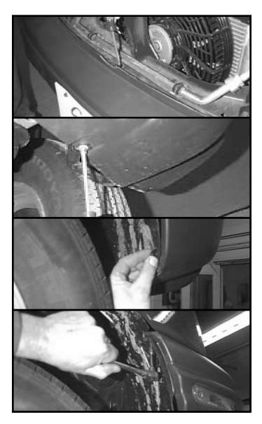
3. Remove bumper cover by removing plastic push fasteners from top side, three bolts from bottom side. Remove one plastic push fastener from inner fender to bumper cover, and one bolt from inner fender to bottom of front fender, on each side.
