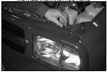
**1.** Remove grill by opening hood and removing plastic push fasteners from top of grill.
