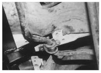
**4.** Remove front bolt from sway bar mounting bracket. **NOTE: Remove front bolts only.**
