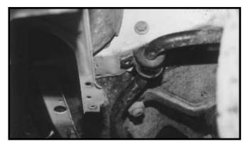
2. Remove front bolt from sway bar mounting bracket. NOTE: Remove front bolts only.
