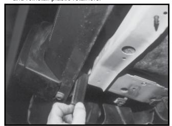
5. Install Frame Nut Plate in the end of frame and align with factory hole.
