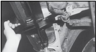
**6.** Slide base plate into position. Base Plate is positioned between sway bar mounting bracket and frame.
