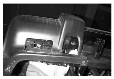
2. Remove left and right plastic bumper extensions, two fasteners on lower side and two attaching to fender on inside.
