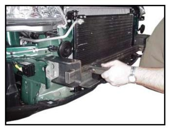
8. Slide base plate on frame horn until the top two bolt holes a lined up on each side.
