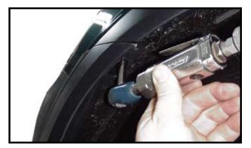
**3.** Remove one screw from each side, facia to fender, by going through wheel well.
