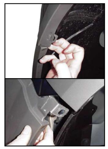
**5.** Pull facia straight down by fender, and release tab on facia (see pictures). Carefully pull facia forward and off.
