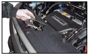
1. Open hood and remove five plastic push fasteners from across top of plastic filler panel.
