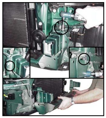
6. Remove facia support tin, four bolts on each side. This assembly and bolts will not be reused. **NOTE:** Some models may have a temp sensor located on tin support, remove clip and relocate.
