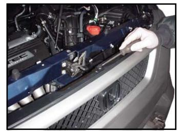
2. Remove nine plastic push fasteners from the top of grill/facia. Note: Facia and grill will be removed as a unit.
