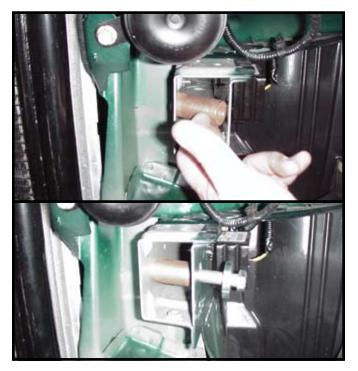
Install spacer bushing inside frame and hold in place with 1/2" x 3-1/2" bolt and heavy frame washer. NOTE: Don't stick 1/2" bolt all the way through so base plate can slide on.
