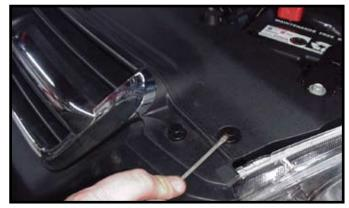
Open hood and remove six plastic push fasteners from across top of grill and facia.
