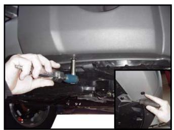
**3.** Remove two bolts from each side from bottom of facia on outside edges and six plastic push fasteners from center, underneath facia front.
