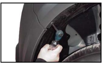
4. Remove one screw from each side of wheel
