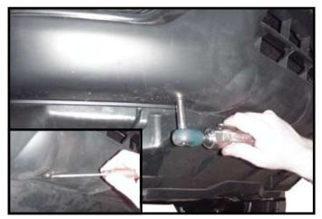
2. Remove two bolts from each side from bottom of facia on outside edges and two plastic push fasteners from center, underneath facia front.
