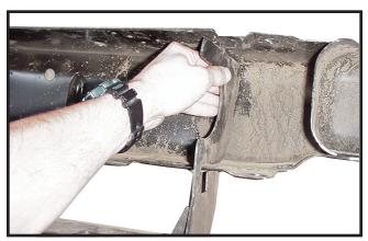
7. Remove plastic panel from inside of bumper. This will not be reused.
