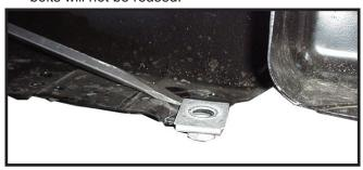
**6b.** If not equipped with tow hooks, remove nut clips from bumper. Nut clips will not be reused.
