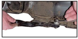
**6a.** After bumper is off, remove both tow hooks, if equipped, from bottom side of bumper. Tow hooks and tow hook bolts will not be reused.
