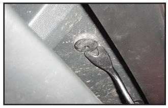
**3.** Remove four plastic push fasteners from middle of facia, under bumper.
