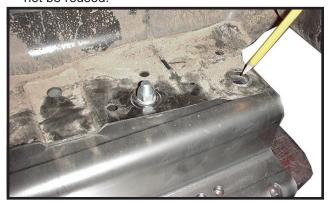
8. Bolt base plate to bottom side of bumper, using two 3/8" x 1-1/4" bolts, 3/8" lock washers and 3/8" nuts. Tighten these bolts when large hole in base plate is centered with large hole in bumper.
