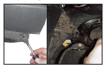
4. Remove one push fastener from each side at bottom of facia, at end of air dam. Also, one push fastener from each side, inside of facia to bumper. Unplug fog lights if equipped and carefully pull facia straight off.
