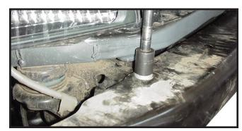
**5.** Remove bumper by removing large bolt from top side, one on each side.
