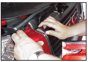
1. **GMC Envoy:** Open hood and carefully pull grill on top to release. Carefully pull tab on bottom of grill forward while pulling up on grill. Rest grill on top of engine compartment if equipped with headlight washers.
