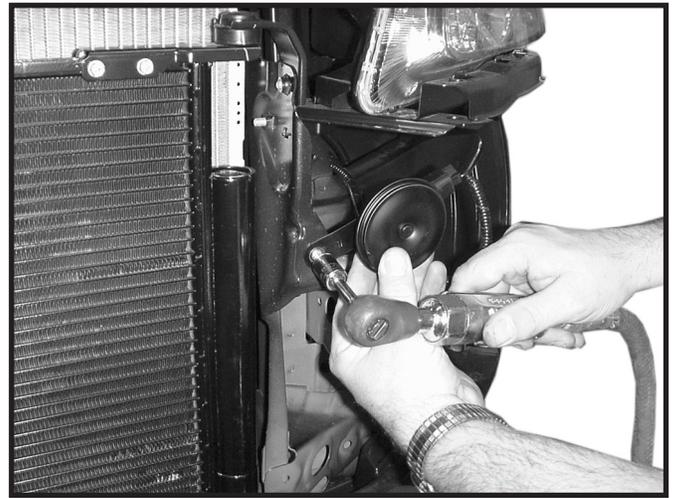
6. Relocate horn on each side, from straight down to outwards. Horn wiring clip will have to be removed from its hole so horn can be loosened and turned according to picture.
