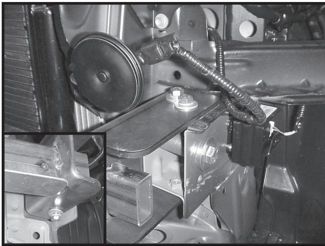
9. Install two 8mm-1.25 x 25mm bolts, 8mm lock washers and 8mm fender washers on top of each side and one 8mm-1.25 x 25mm bolt, 8mm lock washer and 8mm fender washer on bottom of each side. Do not tighten bolts yet. Put 1/2" bolt all the way through other side of base plate and install 1/2" lock washer and 1/2" hex nut. Tighten 1/2" bolts first then tighten 8mm bolts.
