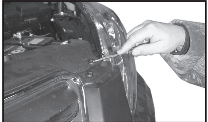
1. Open hood and remove six plastic push fasteners from across top of grill and fascia.
