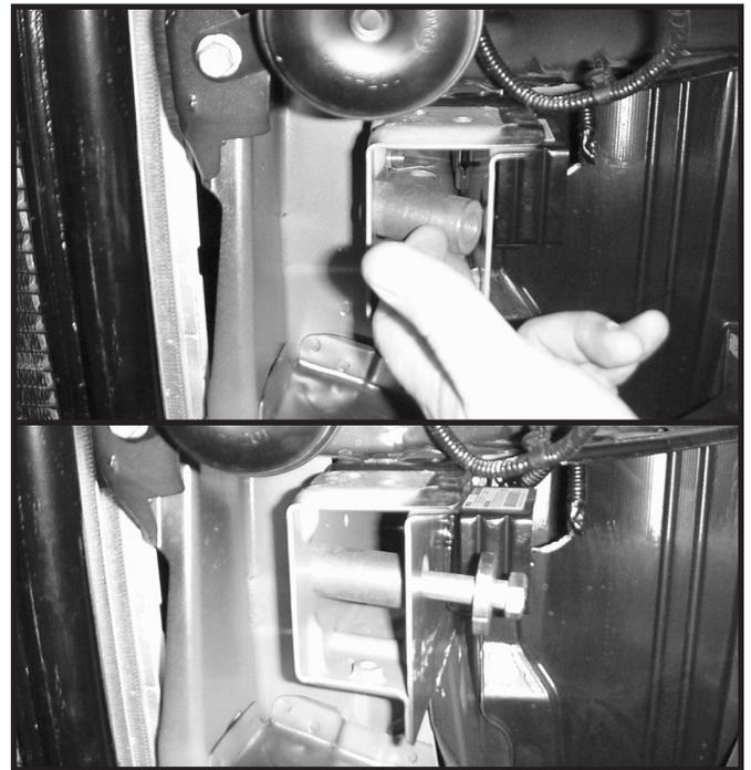
7. Install spacer bushing inside frame and hold in place with 1/2" x 3-1/2" bolt and heavy frame washer. **NOTE:** Don't stick 1/2" bolt all the way through so base plate can slide on.
