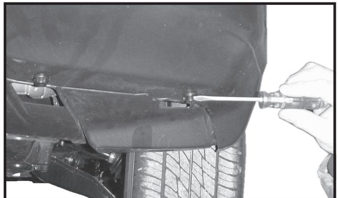
2. Remove six plastic push fasteners from underneath fascia front.
