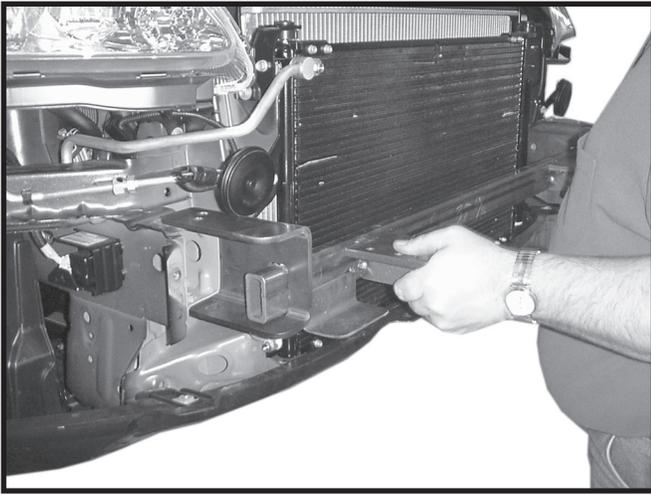
8. Slide base plate on frame horn until the top two bolt holes are lined up on each side.
