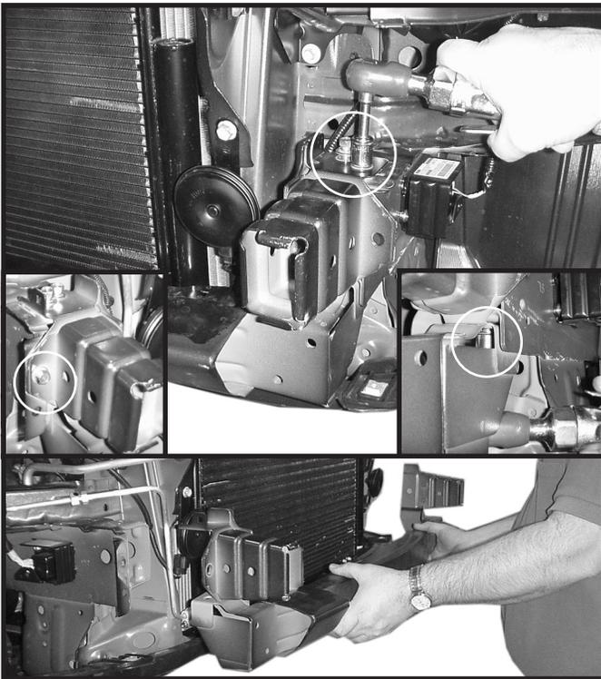
5. Remove fascia support tin, four bolts on passenger's side and three bolts on driver's side. This assembly and bolts will not be reused. **NOTE:** Some models may have a temp sensor located on tin support, remove clip and relocate.
