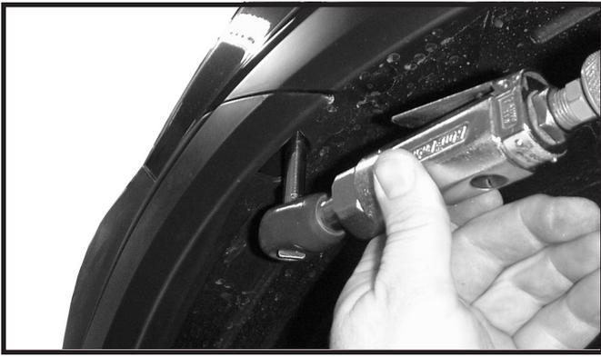
3. Remove two screws from each side, fascia to fender, by going through wheel well.
