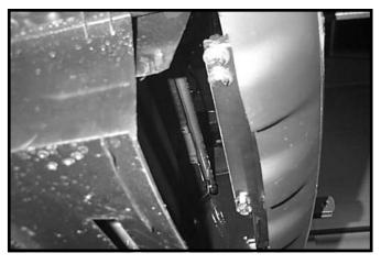
5. Put nuts on the two inside bumper bolts. Do not tighten yet.
