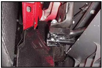
2. Remove bolts that hold right and left tow hooks, two vertical bolts and one horizontal bolt. These bolts maybe very difficult to remove, care should be taken. Tow hooks and bolts will not be reused.
