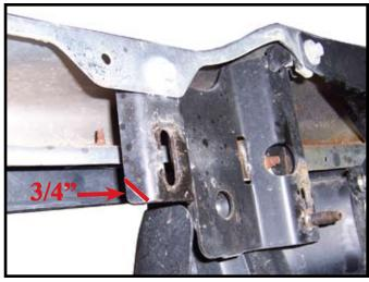
**3.** Trim the bumper mount as shown 3/4" up on each side and remove the retainer washer from the inside two bumper bolts
