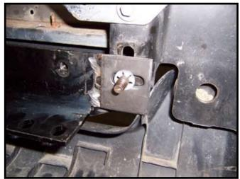
**4.** Install base plate bracket through grill opening and install the provided retainer washers (#04174) over the baseplate. Install 2 heavy washers (07908) over the outside bumper bolts. With an assistant put the bumper and baseplate up as a unit and start the outside two nuts on the bumper bolts. Do not tighten yet.
