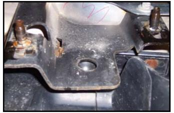
1. Unplug fog lights if equiped and remove the four nuts that hold the bumper on and remove the bumper.
