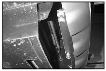
Install 1/2" x 1-1/2" bolts with flat washers from bottom up, two on each side. Secure with 1/2" lock washers and 1/2" hex nuts. Bumper and baseplate may have to be pushed up to start bolts. Do not tighten yet. We require that "LOCTITE. Blue" be used on all bolts.
