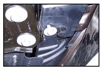
3. Remove one screw and one plastic push fastener from bottom side of facia, on each side.
