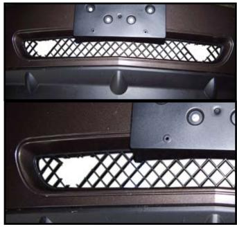
11. Cut lower facia grill as shown in picture. NOTE: Count the diamond pattern in picture for pattern. Trim to fit as desired..
