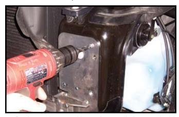
8. Put base plate up with one bumper bolt on each side. Make sure base plate is aligned with matching holes and tighten each bolt. Drill 5/16" hole on each side using base plate as template as shown in picture. Install 5/16" x 1" bolt, lockwasher, and nut thru drilled hole on each side and tighten. Remove previously installed bumper bolts. NOTE: Use LOCTITE. Blue on all bolts.
