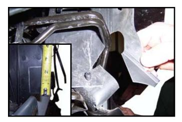
**6.** Plastic behind cooler lines will have to be cut as shown by the white lines in picture. With the palm of your hand, push cooling lines back, also notch on drivers side for clearance of base plate.
