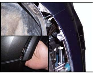
3. Remove one screw on each side from facia to fender and one screw from bottom of facia, unclip wheel well trim, pull facia straight out by fender and partially pull off facia and unplug lights and set facia aside. NOTE: socket and extension will be needed to reach screw.
