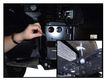
10. Install nut strip thru each side of bumper and align with drilled holes. Fasten using 3/8" x 3" hex bolts and lock washers, and tighten bolts. NOTE: Use supplied shim between baseplate and bumper if needed.
