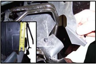
7. Plastic behind cooler lines will have to be cut as shown by the white lines in picture. With the palm of your hand, push cooling lines back, also notch on drivers side for clearance of base plate.
