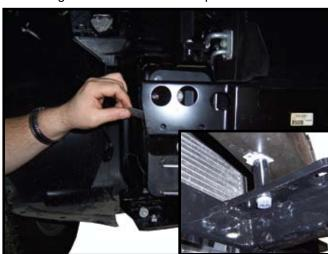
9. Install nut strip thru each side of bumper and align with drilled holes. Fasten using 3/8" x 3" hex bolts and lock washers, and tighten bolts. NOTE: Use supplied shim between baseplate and bumper if needed.
