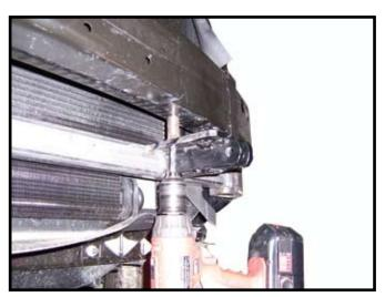
9. Install bumper using previously removed bolts, reinstall rubber filler panel flaps back on bumper with plastic push fasteners. Drill 3/8" hole into bottom of baseplate thru bushing and into bottom of bumper on each side.
