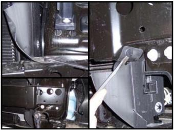
**4.** Remove two plastic push fasteners on each side from top and bottom of bumper (rubber filler panel). Remove five bolts on each side of bumper and remove bumper.
