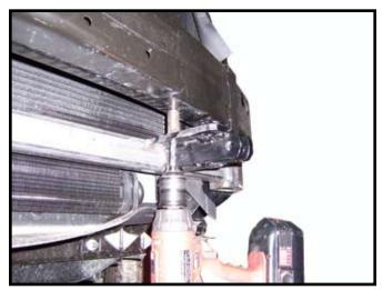
8. Install bumper using previously removed bolts, reinstall rubber filler panel flaps back on bumper with plastic push fasteners. Drill 3/8" hole into bottom of baseplate thru bushing and into bottom of bumper on each side.
