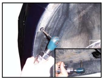
2. Remove five inner fender screws and two more underneath inner fender front extension, on each side.
