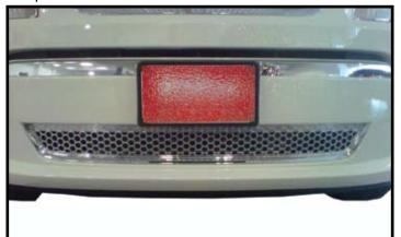
**Denali Only** Cut lower facia by finding center of grill and marking out opening according to measurements in picture. The top of cut out will be even with top of grill as shown in picture. **NOTE:** Best to remove grill insert and mark grill insert with facia on vehicle.
