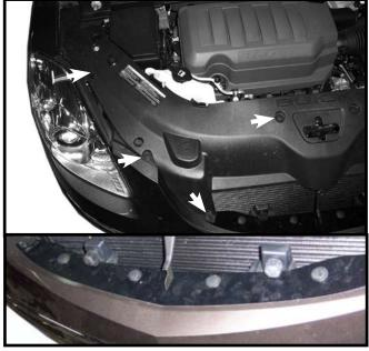
Open hood and remove eight plastic fasteners and remove plastic filler panel. Remove two screws and four plastic push fasteners from top of facia.
