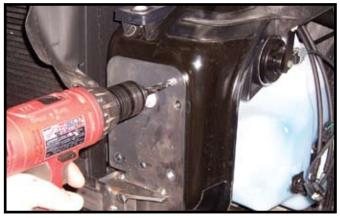
7. Put base plate up with one bumper bolt on each side. Make sure base plate is aligned with matching holes and tighten each bolt. Drill 5/16" hole on each side using base plate as template as shown in picture. Install 5/16" x 1" bolt, lockwasher, and nut thru drilled hole on each side and tighten. Remove previously installed bumper bolts. NOTE: Use LOCTITE. Blue on all bolts.
