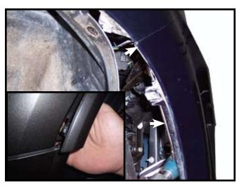
4. Remove one screw on each side from facia to fender and one screw from bottom of facia, unclip wheel well trim, pull facia straight out by fender and partially pull off facia and unplug lights and set facia aside. NOTE: socket and extension will be needed to reach screw.
