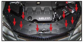
Open hood and remove 6 plastic push fasteners and 4 screws from the panel on top of the grill. Remove center plastic cover and hinge outer covers up and back. Lift outer panel to allow grill to be free.
