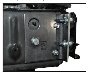
24. Using the supplied fish wire, fish the 3/8" serrated flange bolts up through the hole in the bottom of the frame as was done with the nutstrip. Fasten the bolts in place using 3/8" lock washers and 3/8" nuts. NOTE: Use blue on all bolts and tighten all bolts according to chart on front page.
