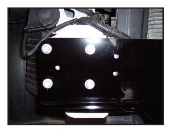
**7.** With and assistant mount the baseplate into place with the bumper bolts.
