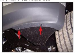
**3.** Remove two screws from the bottom of the facia on each side. Pull out firmly on outer corner of facia from the front of the fender and remove facia.
