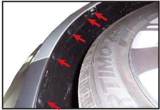
2. Remove three plastic push fasteners and two screws in the front of each fender well.
