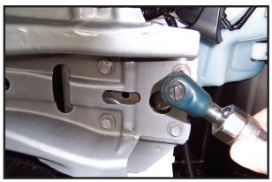
6. Remove four bolts from each side of the bumper and set bumper to the side. **NOTE:** If only three factory bolts are used take factory bolt and use it to tap top inside hole. Then use baseplate as jig to drill hole in bumper to allow bolt to pass through.
