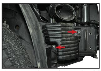
**20.** On passenger side remove the two nuts that hold the airbox baffle in place. Remove baffle and set aside.
