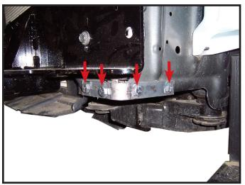
12. Place 3/8 x 1" bolts thru drilled holes and place 3/8" lock washer and 3/8" nut behind frame. NOTE: Use blue **LocTITE** on all bolts and tighten all bolts according to chart on front page.
