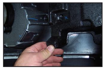
**29.** On the rear of the facia break or cut off the foam tabs from each side to allow facia to fit properly.
