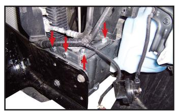
17. Place 3/8 x 1" bolts thru drilled holes and place 3/8" lock washer and 3/8" nut behind frame. NOTE: Use blue LOCTITE on all bolts and tighten all bolts according to chart on front page. Reinstall bolt holding horn on both sides.
