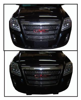
**30.** Reinstall hardware and facia in reverse order as removed. Plug in fog lights if equipped.
