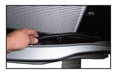
**27.** Route wiring as desired to prevent damage from harness
