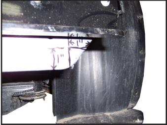
**10.** Cut frame below baseplate on each side as shown in picture.
