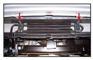
**28. If Equipped** Using the 1/4" x 1 bolts with flat washer and lock washers replace the cooler mounting it to the baseplate in the holes provided as shown.
