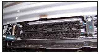
**5. If Equipped:** Remove the cooler from the bottom of the bumper and let hang. **Note:** bolts will not be reused.
