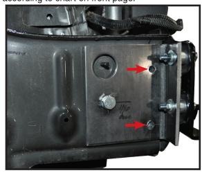
**23.** Drill two 13/32 holes through the outside of frame using the baseplate as a template.
