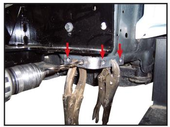
11. Clamp lower bracket to frame as shown. Make sure bracket is flush with bottom of pinch weld. Drill four 13/32" holes using bracket as a template. Repeat on other side.
