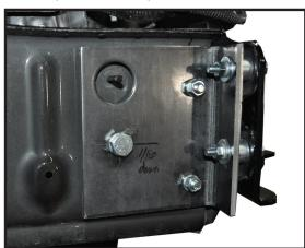
24. Using the supplied fish wire, fish the 3/8" serrated flange bolts up through the hole in the bottom of the frame as was done with the nutstrip. Fasten the bolts in place using 3/8" lock washers and 3/8" nuts. NOTE: Use blue on all bolts and tighten all bolts according to chart on front page.
