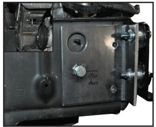
22. Insert 1/2"NC x 1-1/4" bolt and 1/2" lock washer through passenger side bracket and using a nutstrip on inside of frame through hole in bottom of frame as shown in corner picture (leave bolt loose for now). Place 8mm nut, 8mm lock washer, and 8mm flat washer on bolts that come through front of bracket and tighten. Once front nuts are tight then tighten 1/2" bolt. NOTE: Use blue **L@CTITE** on all bolts and tighten all bolts according to chart on front page.
