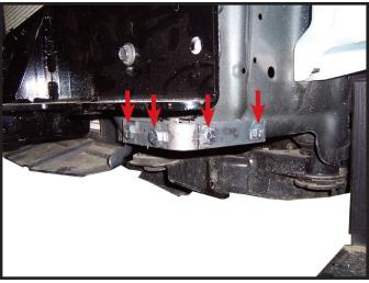
12. Place 3/8 x 1" bolts thru drilled holes and place 3/8" lock washer and 3/8" nut behind frame. NOTE: Use blue **LOCTITE**on all bolts and tighten all bolts according to chart on front page.
