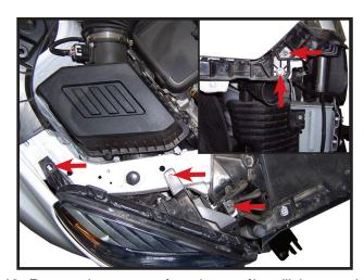
13. Remove three screws from the top of headlight assembly and two from the side (as shown in inserted picture). Pull headlight out and rest on engine. NOTE: Some headlights have a hidden tab holding light to fender. Headlight is removed for ease of drilling.
