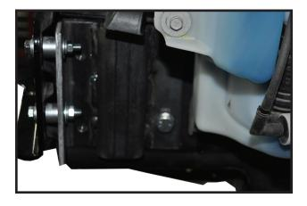
**26.** Instal the driver side bracket in the same ways as on the passenger side. Follow step 21-24 for order of how to install bracket.
