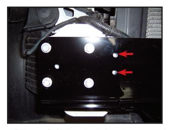
**8.** Drill two 13/32" holes using the baseplate as a template on each sides.
