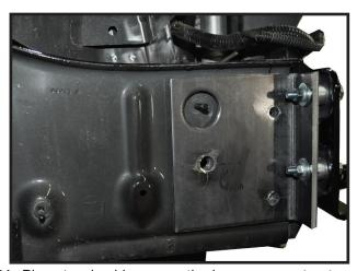
21. Place two bushings over the bumper mount nuts and place passenger side bracket tight to frame and bumper mount. Insert 8mm-1.25 x 50mm bolts, 8mm lock washers, and 8mm flat washers through bumper and passenger bracket. NOTE: Use blue **LOCTITE**<sup>®</sup> on all bolts and tighten all bolts according to chart on front page.
