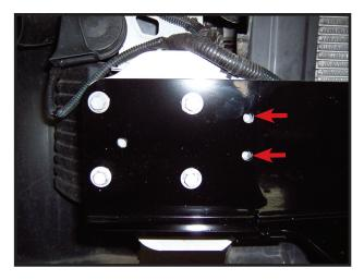
9. Place 3/8 x 1-3/4" with 3/8" flat washers thru drilled holes and place 3/8" flat washer, the 3/8" lock washer and 3/8" nut behind the bumper mount. NOTE: Use blue LOCTITE on all bolts and tighten all bolts according to chart on front page. Minor trimming of the bumper may be required to let the washers in the front Lay flat against the baseplate.
