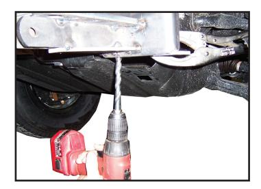
**10.** On drivers side slide baseplate into position and clamp. Drill two 1/2" holes on inside using baseplate as template. Insert nut plate, three 1/2" bolts and washers.
