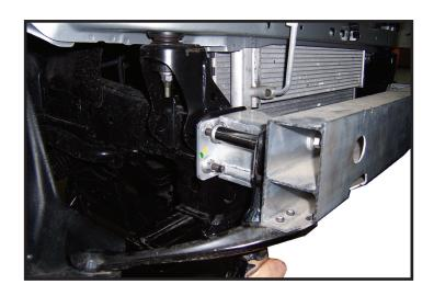
**6.** Remove three nuts on each side of bumper and set bumper aside for later reinstallation.
