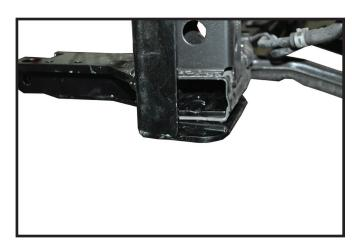
**10.** Place nut plates in tubing over previously drilled holes and slide baseplate pod over bumper studs.
