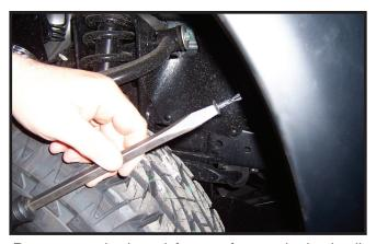
4. Remove one plastic push fastener from each wheel well. NOTE: Turn fastener 1/4 turn to remove.
