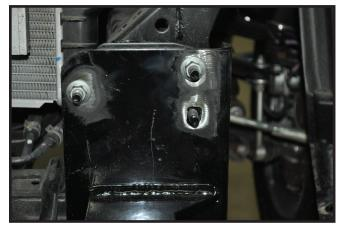
**7.** Place baseplate pods on bumper studs and fasten with factory nuts while pushing pod tight to bottom of frame.
