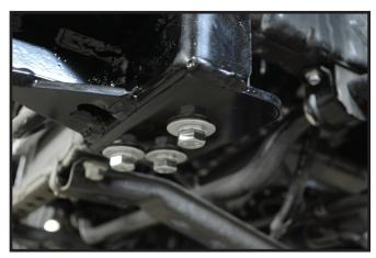
**12.** Insert 1/2" x 1-1/2" bolts with 1/2" flat washers and 1/2" lock washers. Tighten nuts that hold bumper. NOTE: Use Blue **L@€TITE**<sub>®</sub> on threads and tighten bolts according to bolt chart on front page.
