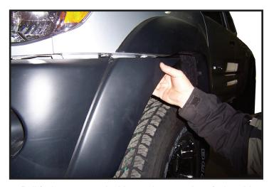
5. Pull facia out on each side to release and set facia aside. If equipped with fender flairs remove one bolt from underneath flair and carefully pull off. On late model vehicles filler panel below head light will also be removed as facia is removed.
