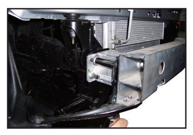
7. Remove three nuts on each side of bumper and set bumper aside for later reinstallation.
