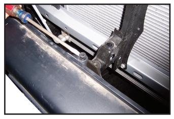
2. Remove three plastic push fasteners from under grill.
