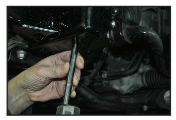
**8.** Transfer punch the bottom three holes of each pod then remove pod.
