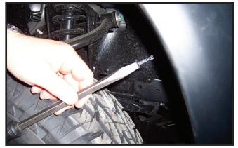
5. Remove one plastic push fastener from each wheel well. NOTE: Turn fastener 1/4 turn to remove.
