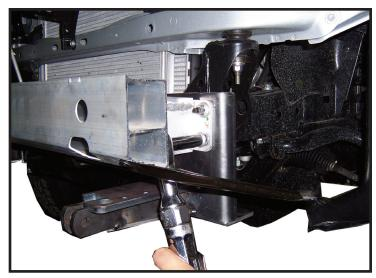
**11.** Slide bumper over baseplate brackets and tighten all bolts.
