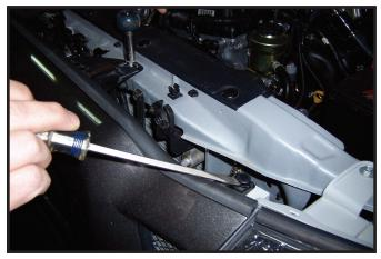
Open hood and remove two screws and two plastic push fasteners from top of grill and two or three plastic push fasteners from bottom, one on each side and one in middle, set grill aside. NOTE: Late model vehicles grill is attached to facia do not remove at this time.
