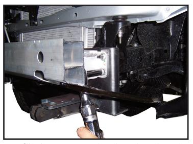
**11.** Slide bumper on to studs and over baseplate pod. loosely tighten nuts.
