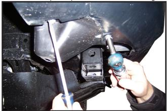
**3.** Remove four plastic push fasteners from under bumper and two screws on each side.
