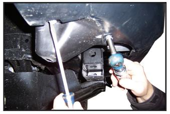
2. Remove four plastic push fasteners from under bumper and two screws on each side. For late model vehicles remove six screws and no push fasteners.
