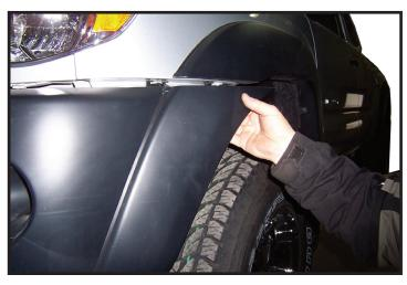
6. Pull facia out on each side to release and set facia aside. If equipped with fender flairs remove one bolt from underneath flair and carefully pull off.
