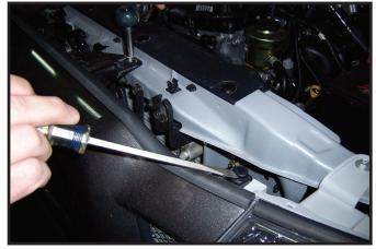
1. Open hood and remove two screws and two plastic push fasteners from top of grill and two plastic push fasteners from bottom on each side, set grill aside.
