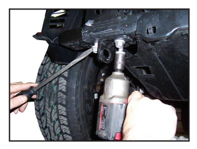
8. Remove end caps and tie down bracket or tow hook on some models. Bolts from end caps will not be reused. Bolts from tie down brackets will be reused.
