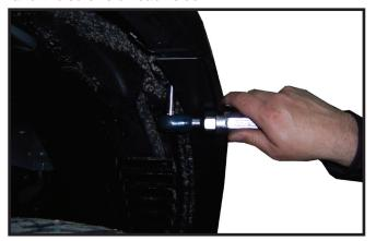
**4.** Remove one screw on each side that connects facia to fender.
