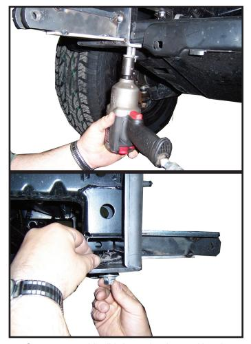
9. On passenger side slide base plate into position, insert two bolts from tie down brackets and one 1/2" bolt and nut strip. **NOTE:** Use Blue **L@€TITE**® on threads and tighten bolts according to bolt chart on front page.
