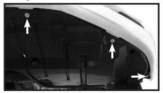
3. From under facia remove three screws from each side.
