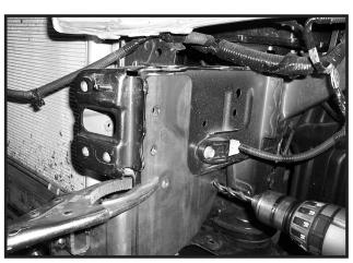
9. With and assistant place the base plate around outer frame and clamp into place butted up to top lip of the frame and the bumper mount as shown. Use the baseplate as a template and drill four 13/32" holes in each side.
