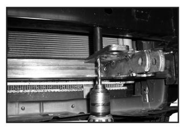
**12.** Using the baseplate as a template drill a 13/32" hole through the bumper.
