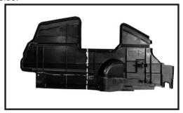
**7.** Trim air dam on each side of the radiator as shown to clear baseplate.
