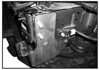
10. Place two 3/8" x 1-1/4" bolt with flat washers in the top two holes from the inside of the frame with two lock washers and nuts. For the lower two holes place two 3/8" X 1-1/4" bolts with flat washers on the outside and 3/8" lock washers and nuts on the inside of the frame lip. NOTE: Use blue **LOCTITE**® on all bolts and tighten all bolts according to chart on front page.
