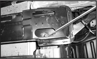
13. Place two 3/8" x 3-1/2" bolts with 3/8" washers lock washers and 3/8" nuts through holes that were drilled. in step 12 and place the nut strip from the end of the bumper. NOTE: Use blue **LOCTITE**<sub>®</sub> on all bolts and tighten all bolts according to chart on front page.
