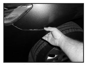
4. To remove the facia pull out firmly from the corner in the wheel well. Pull straight forward with a slight rotation up to clear center mount on top of radiator. Note: Unplug fog lights if equipped.
