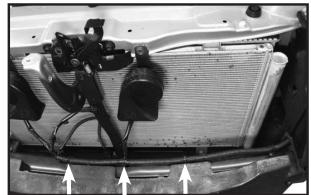
**5.** Remove wiring harness from bumper by prying out the three plastic fasteners.
