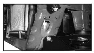
8. Cut the stud bolt off of both sides.
