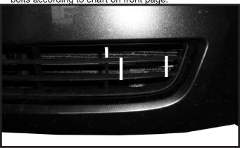
**14.** Cut out pass through for the pull ears of the baseplate. Trim to desired fit and look or remvoe lower section of the grill.
