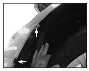
2. On each side remove one plastic 1/4 turn fastener. Then pull back the fender liner and remove one screw attching the facia to the fender liner.
