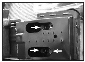
**6.** Remove bumperr by removing three bolts from each side.
