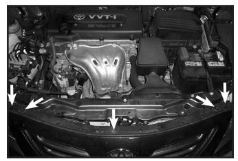
1. Open hood and remove two plastic push fasteners, two phillips head rubber top screws and one bolt attaching the top of the facia to the radiator core support.
