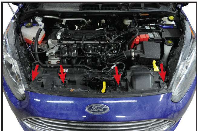
2b. 2014 Remove four plastic push fasteners from top of fascia.
