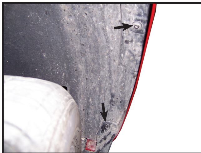
4. On each side remove two screws from fender liner.
