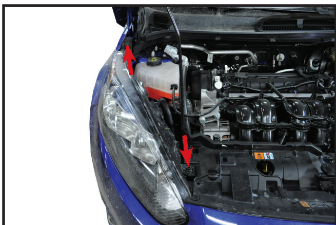
3b. 2014 Remove two screws from each headlight. Remove headlight by pulling up on headlight, unplug wires and set aside.
