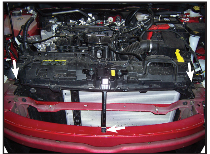
14. Remove three screws from top of bumper.
