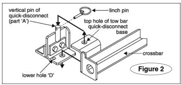
If they are attached too far to the left or the right, the tow bar will not be centered on the towed vehicle, which will cause excessive tire wear and other consequential, non-warranty damage.
