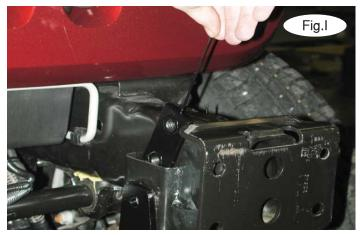
5. Working on the driver's side, place the main receiver brace over the end of the frame rail (Fig.H). Place one of the supplied 3/16" x 1½" x 3½" threaded backing plates with wire through the opening to the inside edge of the frame rail (Fig.I). Using the two supplied ½" x 1¼" bolts and lock washers, bolt through the driver's side main receiver brace, frame rail and into the threaded backing plate with wire (Fig.J).
