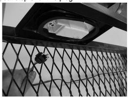
Cover wires with black tubing and secure the harness with cable ties to the bottom of the tray.
