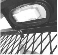
5. Plug the harness into the back of the tail lamp housing.
