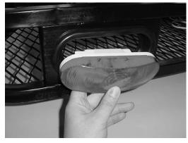
4. Route the 3-way plug with a Yellow wire from under the cargo tray up through the steel grate directly behind the tail lamp housing on driver side of the cargo tray.
