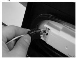
6. Route the 3-way plug with Green wire under the cargo tray over to the passenger side tail lamp. Repeat step 5 for this plug.
