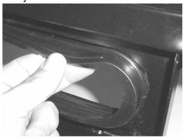
3. Firmly press tail lamp housings into grommets on both sides of cargo tray.
