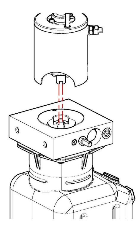
Pump # 2532, 2542 showing motor shaft slot and pump coupler alignment.
