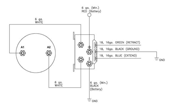
Electrical Connections: Motor # 2751 and contactor # 2994 used on pump #s 3040, 3041 and 3043
