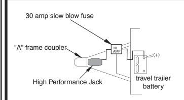
Connect the lead-wire directly to the positive (+) lead of the travel trailer's battery using a twelve (12) gage wire. Be sure the connection is a good one.
