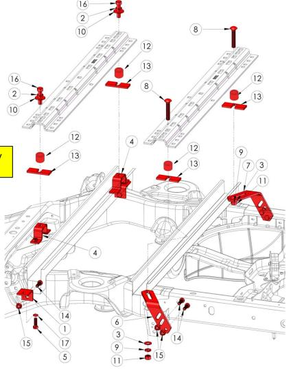
Do not install mounting rails over plastic bed liners. Plastic bed liners must be cut out of the way to provide metal to metal contact. Mounting rails may be installed on spray in liners. Check with liner mfg's for cure time. Use only bolts nuts and washers supplied.
