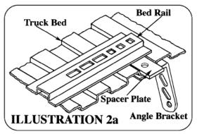
5. Position the angle brackets (#2) under the bed, at the rear attachment and align with the 5/8" carriage bolts (#6) protruding down through the bed. Slide tube spacers (#1) into the forward under bed hat section from the open end in each wheel well.
