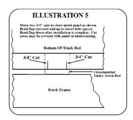
6. Moved the installed angle brackets so that they rest tightly against the flat side of the truck frame and underneath surface of truck bed. Drop 5/8" carriage bolts (#6) down through bed rails and angle bracket.
