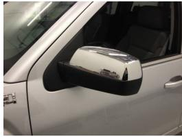
Remove masking tape, place Putco mirror cover in factory location and press firmly until all snaps are fully engaged. Repeat steps 2-5 on Passenger side
