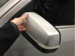
4. Pull up and out on loose mirror cover until cover is removed
