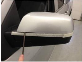
3. Use flat head screw driver to pry on the lower portion of the factory mirror cover until the clips release
