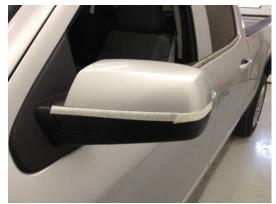
Place masking tape along bottom edge of the factory mirror cover. (Driver side is pictured)
