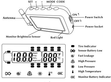
Pressure Unit: BAR, PSI, Kpa, Kgf/cm<sup>2</sup> Temperature Unit: C, F
