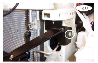
16. Place the driver's side rear brace over the hole you exposed in the previous step, and using a supplied 14mm x 1.5 x 80mm bolt with thread lock, bolt through the rear mounting point and subframe and lock washer.
