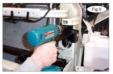
19. Using a 10mm drill bit and the side mounting point on the upper support as a template, drill a 10mm hole through the core support (Fig.V).
