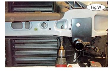
ceiver brace as a template, drill up through the bumper core (Fig.W). Bolt up through the main receiver brace and bumper core using a  $\frac{1}{2}$ " x 1 $\frac{3}{4}$ " bolt and finish with a 3/16" x 1 $\frac{1}{2}$ " x 3" backing plate,  $\frac{1}{2}$ " lock washer and nut.
