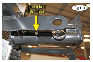
23. On each side, insert the removable front bracket arm into the front receiver 90 degrees from its final towing position, depressing the spring-loaded pin against the receiver (Fig.CC). Now, twist back 90 degrees until the spring-loaded pin snaps into place in the notch on the receiver, locking the arm into place in its final towing position (Fig.DD).
