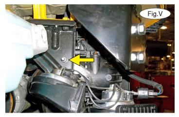
small tabs on the side of the horn mounting bracket. On the driver's side only, remove the electrical connector shown in Figure N and then reattach the horn bracket in its pre-existing hole in the radiator support. Then, remount the passenger side horn using Figure O as a reference. Remount them so that they do not contact the bracket. Loosen the nut attaching the horns to their mounting brackets to swing them out of the way as necessary to accomplish this.
