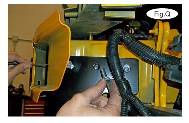
bolt through the center hole of the support bracket and into the backing plate. Repeat for the remaining two outer holes on each side after removing the bolts.
