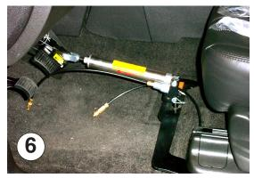
*Note*: some 2008 models with adjustable pedals may not require the adjusting arm on the air cylinder (Fig.1). Instead, it will mount directly to the mounting post, as shown in Figure 6.
