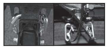
**Step 3.** Insert receiver pin through receiver until pin passes through. Secure pin with the Receiver hair pin. Crisscross safety cables underneath pivot assembly and attach to chain anchors on towing vehicle.
