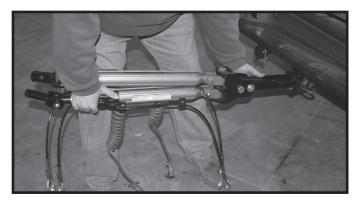
Step 2. Insert the Dominator into a Class III or IV hitch.
