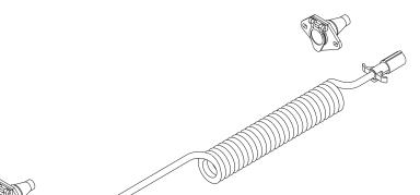
NOTE: To be used with optional Light Bar, the ends will have to be cut off light bar harness. This end will then need to be wired to the receptacle of the auxiliary lighting kit.
