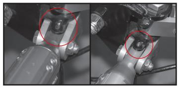
**Step 4.** Now take the bottom leg and lift up high enough for storage pin to clear under storage plate. Turn leg under storage and push leg down so pin locks into plate. Repeat for top leg.
