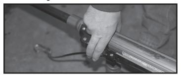
**Step 2.** Use the latch trigger handle to release the connecting legs between the two vehicles by pressing down on the latch trigger handle. One connecting leg may have more pressure against it, do that one first.
