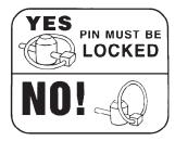
Quick-lock pin must be closed properly. Fold ring of Quick-Lock Pin to the side of the pin that allows ring to snap against pin. If you have folded its ring the wrong way it will not snap against pin.
