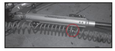
**Step 7.** Leave the electrical cable storage pin (circled above) out for the locking procedure in step 6. When step 6 is completed, position cable on storage rod leaving enough slack, and insert pin.
