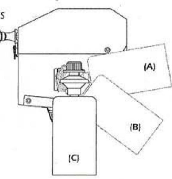
Valve will feel loose and will rotate easily. Even though the valve feels loose, it is designed that way and will not leak. The valve was designed to be loose fitting in order to allow safe, easy installation and removal of the propane canister and so it easily swings without resistance to fit all applications
