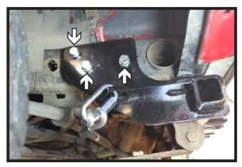
On the passenger side, using a 1/2" drill bit, drill the three (3) holes in the baseplate thru the frame. Install 1/2"-13 x 2-1/2" bolts with lock washers and 1/2"-13 whiz nuts on the inside of the frame. Fully tighten all hardware.
