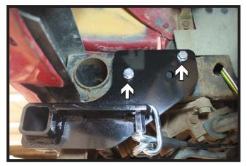
Using a 16MM socket, remove the two
