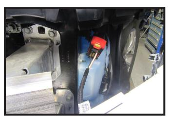
As the fascia is removed unhook the plug on the driver side by pulling out the yellow piece and up on the red part to unhook. Remove fascia and set aside to be reinstalled later.
