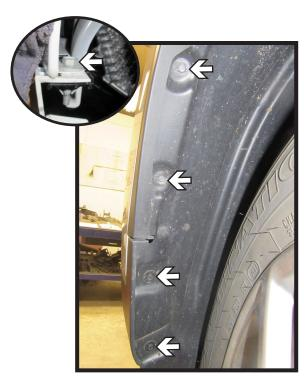
Using an 8MM socket, remove the four (4) bolts from the edge of the wheel well. Pull back the wheel well cover, using a 10MM socket, remove the bolt behind the trim (inset). Do this on both sides of the vehicle.
