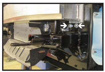
8. Slide the baseplate into place and start the two (2) 10MM bolts with 3/8" flat washers and lock washers on the bottom of the bumper. Do this on both sides of the vehicle.
