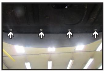
4. Using a 10MM socket, remove the four (4) bolts on the underside of the vehicle.
