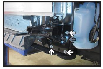
9. Insert the three (3) existing 10MM bolts with 3/8" flat washer and lock washer (white) and one (1) nut (gray). Tighten all hardware fully. Do this on both sides of the vehicle.
