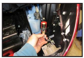
Lift the corner of the fascia up towards the fender and out to release. Continue along under the headlights unsnapping the fascia from the vehicle. As the fascia is removed unhook the plug on the driver side by pulling out the yellow piece and up on the red part to unhook. Remove fascia and set aside to be reinstalled later.
