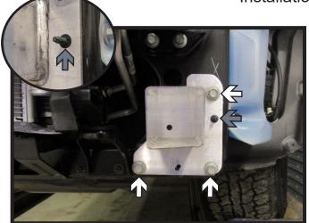
Using a 15MM socket, remove the three (3) bolts from the frame extension. Using a 10MM socket, remove the nut (gray) from the frame extension. Do this on both sides of the vehicle. Remove frame extension, it will not be reinstalled. **Note:** Some models my have a clip that needs to be removed instead of a nut (inset).
