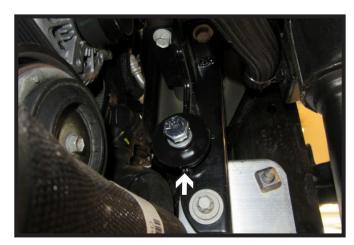
From the backside install the 1/2" x 5" bolt with lock washer and 1/4" x 2" DIA washer. Do this on both sides of the vehicle.
