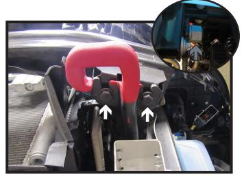
Using a 16MM socket, remove the two (2) bolts (white) from the underside of the tow hook. Using a 30MM socket, remove the nut (gray) from the backside of the tow hook (inset). Do this on both sides of the vehicle. Remove tow hooks and set aside, they will not be reinstalled.
