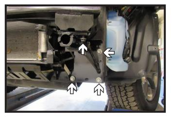
Slide the baseplate into place and install the four (4) existing 10MM bolts. Tighten the bumper bolt first, then tighten the remaining three (3) bolts. Do this on both sides of the vehicle.
