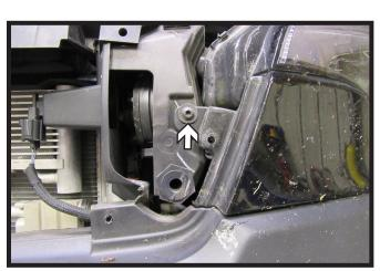
2. Using a T27 Torx, remover the one (1) screw from behind the fascia cover. Do this on both sides of the vehicle.
