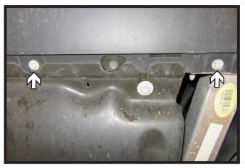
Remove the one (1) rivet (gray) from the underside corner of the fascia. Using a 10MM socket, remove the two (2) bolts (white) from the underside of the fascia. Do this on both sides of the vehicle.
