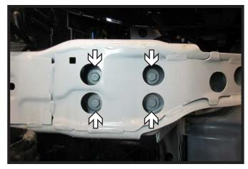
7. Using a 13MM socket, remove the four (4) bolts from the bumper. Do this on both sides of the vehicle. Unsnap the wire loom from the bumper and remove bumper. The bumper will not be reinstalled later but will be replaced by the baseplate.
