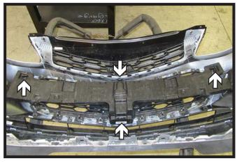
Remove the foam piece from the back side of the fascia by releasing the four (4) clips holding it in place. This will not be reinstalled later.
