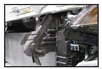
Using a utility knife remove the plastic piece as indicated. Do this on both sides of the vehicle.
