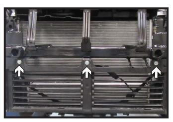
14. Lift shutter housing back into place and attach to the baseplate using three (3) 1/4" bolts with flat washer and nylon lock nut. Note: The middle hole may need to be drilled out with a 1/4" drill bit on the shutter piece.
