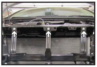
13. Reinstall the three (3) front support brackets by placing bottom into slots on the baseplate and reinstalling existing bolts at the top.
