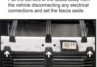
Using a 7MM socket, remove the three (3) bolts from the shutter housing. Let shutter hang loose.
