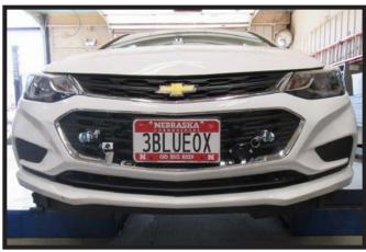
16. Hold the fascia as close to its original position, mark and trim the fascia around the convenience links and attachment tabs. Reinstall the fascia and fascia cover
