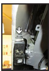
2. Using a T15 Torx, remove the two (2) screws from the edge of the wheel well in front of the tire. Next, pull the cover back. Using a 7MM socket, remove the one (1) bolt from under the cover. Do this for both sides of the vehicle.
