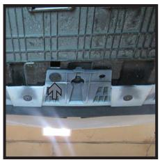
3. Using a 7MM socket, remove the six (6) bolts (white) from the underside of the vehicle. There are three (3) on each side of the car. Remove the one (1) push pin (gray) from the center of the underside.
