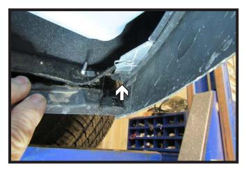
Pull the plastic piece down and using a 7MM socket, remove the one (1) bolt.
