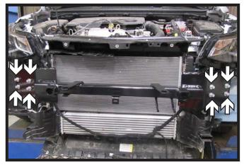
11. Slide the baseplate into place and start the eight (8) 8MM bolts, four (4) on each side, with flat washer and lock washer. Then tighten fully.
