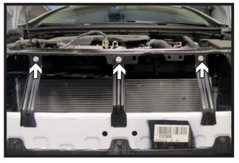
Using a 10MM socket, remove the three (3) bolts holding the support brackets. Remove brackets and set aside to be reinstalled later.
