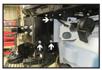
12. Using a 3/8" drill bit, drill out the three (3) holes for the side plate. Be careful not hit any wires while drilling. Then insert the three (3) 3/8" bolts with lock washer and 3/8" whiz nut with wire. Do this on both sides of the vehicle.
