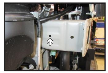
7. Using a 3/8" drill bit, drill out the back hole in the frame on the passenger side of the vehicle.
