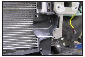
8. Measure down approximately 3-1/2" from the top of the shielding and cut thru the plastic shielding. Discard the upper portion of the shielding. Do this on both sides of the vehicle.
