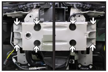
Using a 13MM socket, remove the eight (8) bolts from the bumper. Remove bumper and set aside to be reinstalled later.
