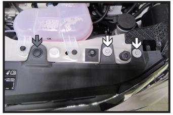
1. Using a 10MM socket, remove the four (4) bolts (white) from the top of the fascia. Then remove the two (2) push pins (gray).
