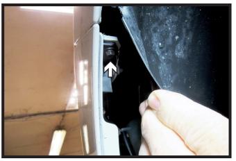
3. Pull back the wheel well liner. Using a 7MM socket, remove the one (1) bolt from the fascia joint. Do this on both sides of the vehicle.
