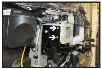
10. Using a 3/8" drill bit, drill the remaining two(2) holes using the baseplate as a guide. Do this on both sides of the vehicle.
