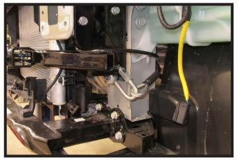
12. Attach the permanent baseplate safety cables to the provided convenience link on the baseplate. The photo above shows the recommended installation of the cables to frame of vehicle. Additional options may interfere with suggested mounting; in this case, secure the cables to a solid piece of the frame as described in the General Information sheet. Be sure the safety cables do not rub against any hoses or moving parts. Do this on **BOTH** sides of the vehicle.
