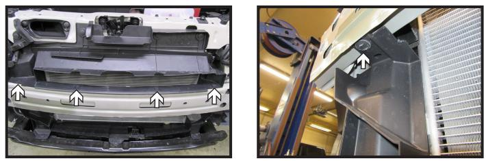
5. Remove the four (4) push pins from the top of the bumper and two (2) from the bottom of the bumper, one (1) on each side.
