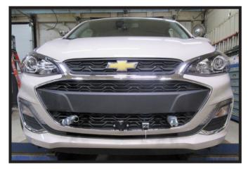
14. Hold the fascia as close to its original position, mark and trim the fascia around the convenience links, attachment tabs and optional breakaway switch. Reinstall the fascia and reconnect all electrical.
