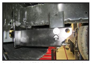
5. Install the 1/2" bolt with hardware into the rear baseplate hole thru the extension. Fully tighten all hardware. Do this on both sides of the vehicle.
