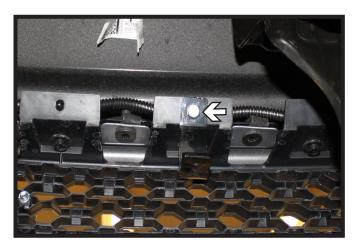
7. **Optional Breakaway:** On the inside of the lower grill remove the push pin at the desired location and install the bracket with the 1/4" hardware provided. Trim the lower grill and install the breakaway to the bracket with the 1/4" hardware provided.
