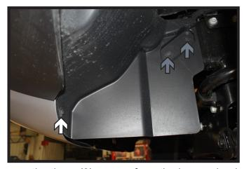
1. **Rebel Models Only:** Using an 8MM socket, remove the three (3) screws from the lower wheel well liner (white). Then remove the two (2) push pins (gray) and set the liner aside. Do this on both sides of the vehicle.
