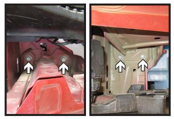
Using a 12MM socket remove the four (4) bolts attaching the bumper to the frame. Do this on both sides of the vehicle. Remove bumper and set aside, it will not be reinstalled later.
