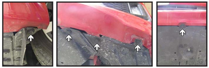
3. Remove the ten (10) push pins from the underside of the vehicle, five (5) on each side. Then remove the fascia and set aside to be reinstalled later
