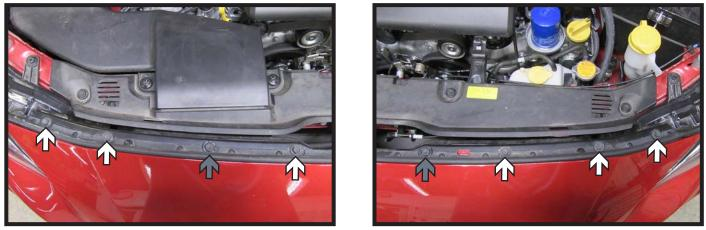
1. Using a 10 MM Socket remove the six (6) bolts (white) and two (2) push pins (gray) from the top of the fascia.
