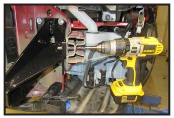
8. Using a 1/2" drill bit, drill a hole through the frame as indicated so that it meets up with the corresponding slotted hole on the baseplate. Do this on both sides of the vehicle.
