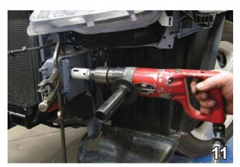
11. **ALL MODELS:** Drill a hole in the frame rail using the 1 1/4" hole saw on both sides. This hole will allow installer to insert nut plates inside of frame rail in steps 13 and 14.
