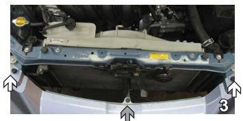
3. **2008 MATRIX:** Using the Phillips screw driver, remove the Phillips screw from the top of the fascia outer edge, both sides. Also remove the push pin from the center (gray arrow).
