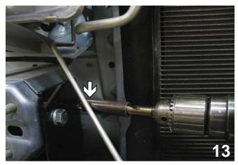
13. **ALL MODELS:** Using the baseplate as a template, drill both holes in the side of frame rail with a 17/32" drill bit. Do this to both sides. Insert nut plates into 1 1/4" drilled hole on outer side of frame rail to align with drilled holes. Tighten the 1/2" hex bolts and lock washer with the 3/4" socket into nut plates. Do this to both sides.
