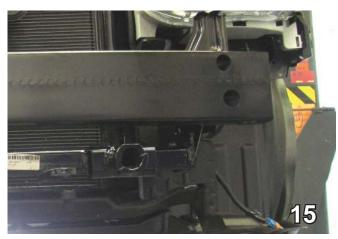
15. **ALL MODELS:** Reinstall bumper bracket, metal bumper and styrofoam. Be sure to reattach wire loom to top of bumper.
