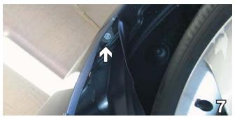
7. ALL MODELS: Remove metric bolt just forward the front tire on upper corner of fascia and inside of wheel well, using a 10MM socket. Do this to both sides. Pull fascia forward, unplug electrical connection to fog lights, and carefully set aside for reinstallation later.
