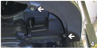
ALL MODELS: Using a 10MM socket, remove two metric bolts just forward of front tire. Do this to both sides and set aside bolts for later reinstallation.
