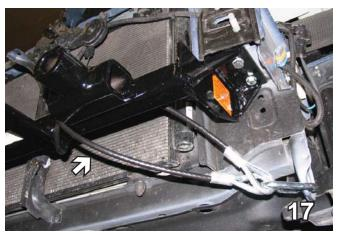
17. **2008 MATRIX:** Attach the permanent baseplate safety cables to a solid piece of the vehicle's frame as in above photos or as close to as possible.
