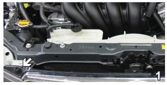
2005-07 MODELS: Using the Phillips screw driver, remove the Phillips screw from rubber bumper, do this to both sides and set rubber bumper aside for later reinstallment.
