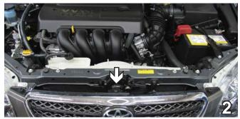
2005-07 MODELS: Remove push pin from top edge of fascia just below hood latch and set aside for reinstallation later.
