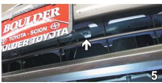
2005-07 MODELS: Behind fascia on bottom of metal bumper, are two push pins to remove from facia's tabs. Remove with flat screw driver and set aside for later reinstallation.
