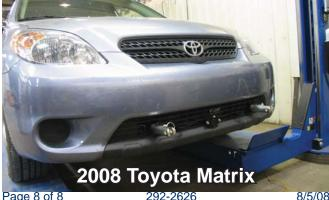
Install the tow bar and safety cables according to the instructions provided in their packages. When demonstrating this to the customer, be sure to include all the contents and packages.
