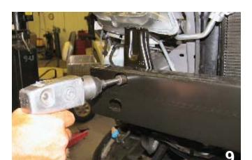
ALL MODELS: Using a 14MM socket, remove four metric bolts from metal bumper and set aside for later reinstallation.
