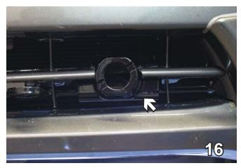
16. 2005-07 MODELS: Hold fascia as close to its original position as possible, mark and cut grill with utility knife to allow baseplate receivers to come through. Plug in fog lights in applicable on back side of fascia and reinstall fascia.
