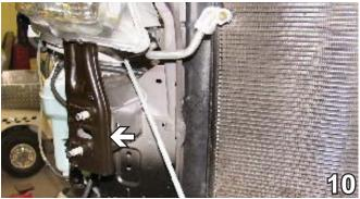
10. **ALL MODELS:** Remove bumper bracket from both sides and set aside.
