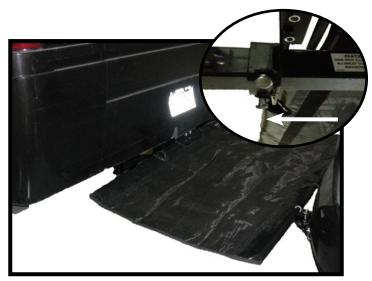
3. Hook up the tow bar to the towed vehicle per the tow bar instructions. Slide the front arm torwards the motorhome along the receiver mount until the screen is tight, then tighten the bolts on the underside to secure in place.
