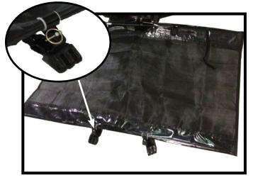
Slide the KarGard<sup>™</sup> II onto the receiver tube of the tow bar, then install the tow bar onto the towing vehicle per the tow bar instructions. Extend the legs of the tow bar until the leg support lines up to the holes in the clamp brackets. Install the 3/16" linch pins to secure together.
