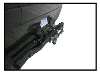
When not in use, roll the KarGard<sup>™</sup> II up and secure with the attached velcro strips.
