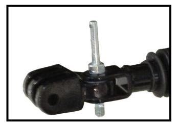
Using the 3/4" Socket and wrench, replace the existing bolts of the tow bar legs with the leg supports and 1/2"-13 essna jam nuts.
