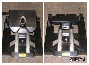
1. Remove clips and pins holding top plate assembly in place and set plate aside.
