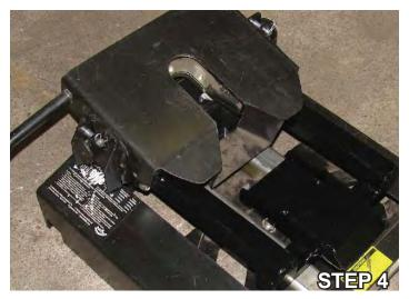
4. Reinstall top plate and secure with original pins and clips. Check top plate movement to assure it is not obstructed by BedSaver.
