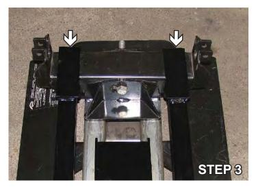
3. Position the BedSaver in the center between both upright arms. Tighten nut and bolt assemblies to 78 ft. lbs then verify free movement of hitchslide mechanism in both directions.
