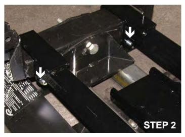
2. Slip BedSaver weldment over hitch crossarm and loosely install the four bolts and nuts as shown.
