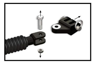
Using a 3/4" socket and wrench, remove the existing 1/2"-13 bolt and 1/2"-13 jam nut from the tow bar leg. Remove the existing lug and washers from the tow bar leg. Do this on both tow bar legs.
