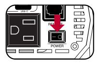
The power inverter is now ready to deliver AC power to your loads. If several loads are to be operated by the inverter, turn them on separately, after the inverter has been turned on. This will ensure that the inverter does not have to deliver the starting currents required for all the loads at once.
