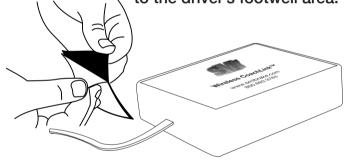
**Note:** For a more hidden installation locate the CoachLink<sup>™</sup> Transmitter under the driver's side dash area and secure it in place with the provided hook and loop fastener.
