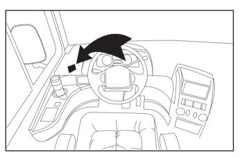
Plug the CoachLink™ Receiver in to an auxiliary 12v plug in the coach dash area.
