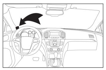
Secure the 900MHz transmitter in place using the provided hook and loop fastener and route the wire around the edge of the dash and down to the driver's footwell area.
