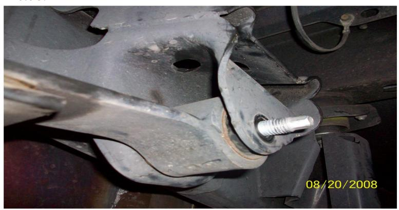
**4.** Using the bolt fisher (**see bolt fishing instructions**) install one 1/2" x 2" hex bolt with one star washer, one flat washer, and one star washer from the backside of the spring hanger into the top hole of tie down receiver. Secure the bolt with two flat washers, one lock washer and one nut. Tighten now. Repeat for driver side installation. (PHOTO 4.1)
