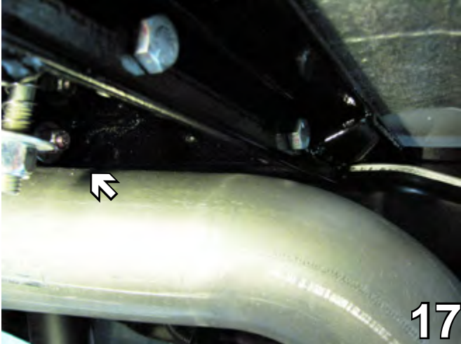
17. Hook the exhaust back up using the existing brackets and existing hangers.
