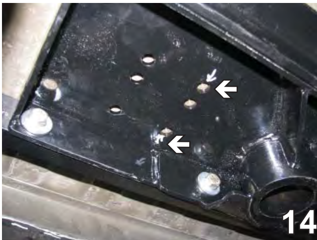
14. Using the cross member as a template, drill with a 19/32" drill bit the two holes for the u-bolts. Do this on both sides.
