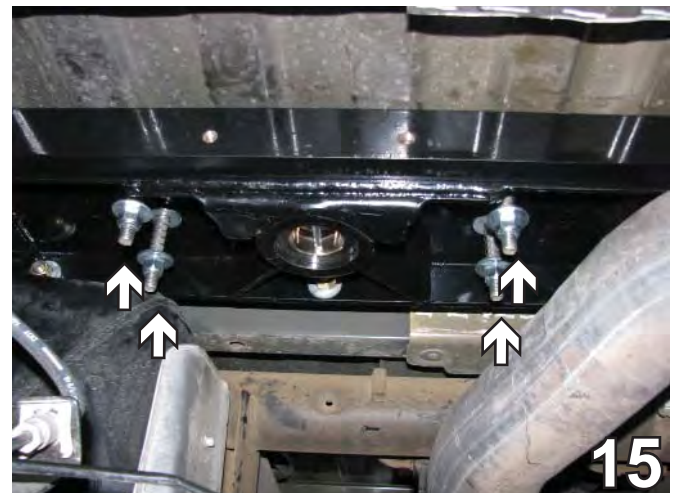
15. Insert the 1/2-13 U-bolts from the top side of the truck bed and attach the 1/2" flat washers, springs, 1/2" flat washers and 1/2-13 lock nuts below.
